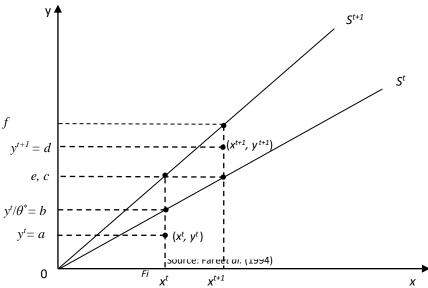
The input-output combination  $(x^t, y^t)$  in terms of distances of technology  $S^t$  can be written as Oa / Ob or  $\|y^t\| / \|y^t / \theta^*\|$ , that is less than 1, therefore, shows inefficient input-output proportion. The best practice output or the highest possible level of productivity under CRS can be achieved if average productivity (y / x) is maximized which also represents observed TFP change (Färeet *al.*; 1994). The MPI (TFP change) is measured as:
